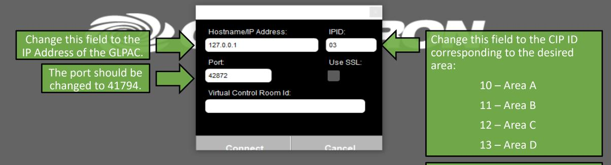
If there are physical TSW panels installed with these CIP ID, the XPanel and the physical panels will mirror each other.
